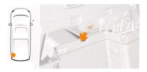
2. Pull the emergency release cable to open the fast charging cover. 3Restore the emergency release cable to the fixed position, and reinstall the left emergency cover of the trunk.
